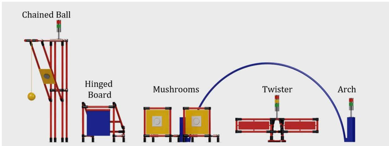
2.8.04 The Hinged Board actuator is a rectangular board hinged at its top. The board must be pivoted so that it triggers a pressure plate, activating the corresponding power-up.
